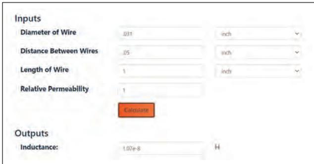
▲ Fig. 5 Many online calculators are available for determining the inductance of parallel wires: This example shows the total inductance of a pair of 1 in. long, 31 mil diameter wires, spaced 50 mils apart. Spacing the wires 100 mils apart will approximately double this inductance.
