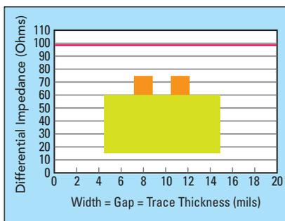
▲ Fig. 8 When trace thickness, line width and gap are the same value, and the plane is very far away, the differential impedance is close to 100 Ohms. Because the fringe fields between the two traces are invariant with the ratio of the dimensions, keeping the ratios fixed means the differential impedance is fixed over all dimensions.
