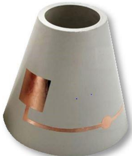
Copper patch antenna patterned directly on TMM substrate
