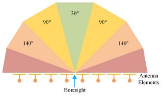
**Figure 5:** A depiction of a linear phased array's gain performance at various angles away from the boresight with green being the highest and red being the lowest.
