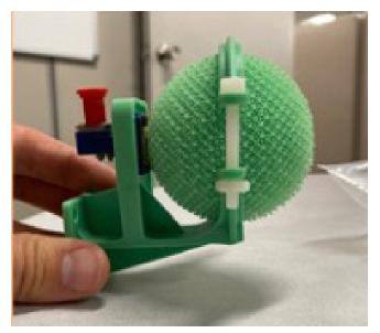
**Figure 17:** GRIN Luneburg lens built using conventional, commercially available photopolymer resin.
