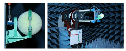
Figure 15: Left - The 3D printed GRIN lens mounted to the fixture in front of the open ended waveguide feed source. Right - The mounted lens affixed to the test rig in the anechoic test range.
