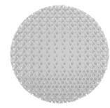
Figure 13: This device cross- section shows how the volume fraction of material reduces radially from the center of the sphere to the surface.
