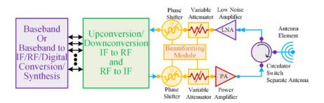
**Figure 6:** A simplified RF frontend (RFFE) for a phased array antenna element that is directly driven.
