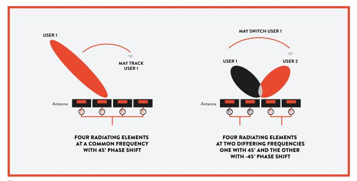
Figure 2: A beamsteering antenna
