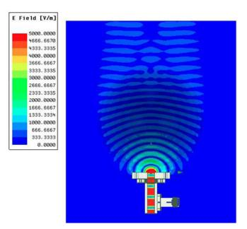
Figure 12: Lens design modeled in Ansys HFSS showing the electric field being focused by the GRIN structure.
