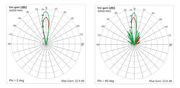
Figure 18: 30 GHz test results for the two lenses. In both charts, the green curve is the Rogers and Fortify printed lens, where the red curve is the comparative lens printed with commercially available photopolymer. Left chart - Phi = 0. Right chart - Phi = 90.
