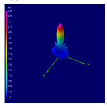
Figure 16: 3D antenna pattern of the printed Luneburg-style lens at 30 GHz.
