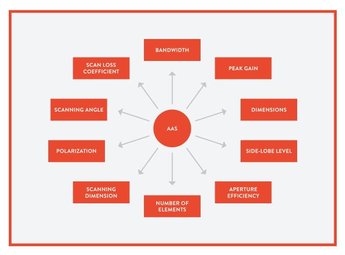
Figure 3: The main figures-of-merit (FOM) for AAS
