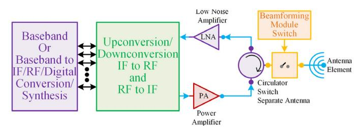
Figure 9: Example dielectric lens switched antenna array signal chain for a single element.
