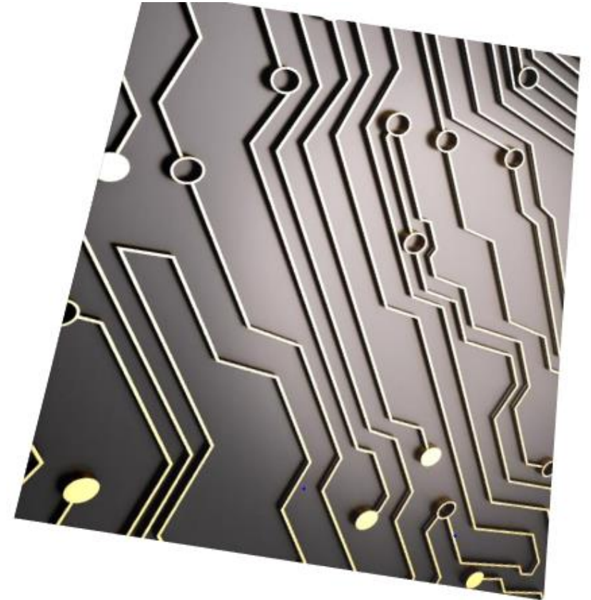
Ratio of height-to-width of the circuit trace impacts signal integrity
