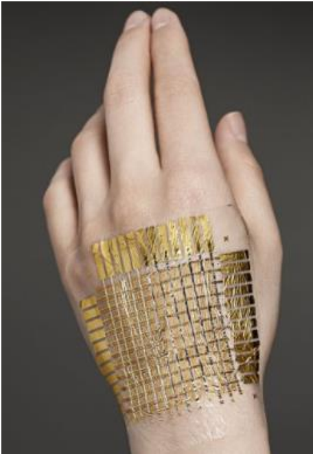
Super light and flexible circuits for wearable computers
